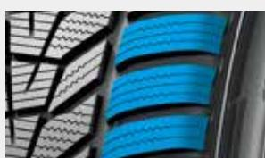
Reduction of the kerf thickness optimizes each block stiffness to achieve advanced dry performance and road holding.
