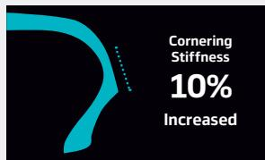
Tire stiffness is essential to be improved to bear the weight of electric vehicles. Hankook's EV Contour Technology increases cornering stiffness by 10% to advance electric vehicle handling performance.
