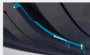
The water pipe kerf placed inside the shoulder block improves performance on wet surface by efficiently transporting water out of the main groove.
