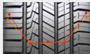
Dry handling performance is improved by the expanded outside shoulder block and increased lateral stiffness. A wider outside shoulder block ensures good dry handling performance, lateral stability, and steering response.
