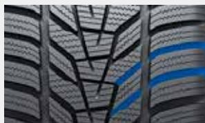
Unidirectional Tread design with gull wing shaped improves the traction and braking performance on snow.
