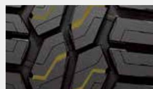
V shaped lateral grooves bite the surface for additional off-road grip.
