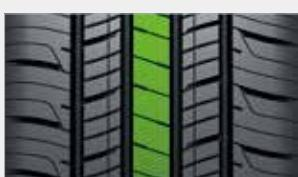
A rigid center rib provides excellent grip for outstanding handling and braking performance.
