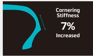
Tire stiffness is essential to be improved to bear the weight of electric vehicles. Hankook's EV Contour Technology increases cornering stiffness by 7% to advance electric vehicle handling performance.
