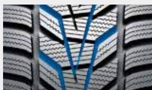
V-shaped pattern efficiently help to distribute water to the side, improving hydroplaning performance.
