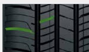
Wide lateral grooves incorporated into the tire's tread ensure hydroplaning resistance for excellent wet handling and braking.
