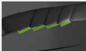
Serrated edge design at the end of the tread block maximises the edge effects and enhances winter driving performance.
