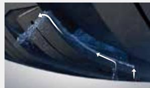
Water pipe kerfs are placed inside the shoulder blocks for water drainage from the main groove, which maximizes grip on wet roads.
