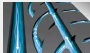
Catalyst to channel water out of the center to the main groove wall effectively. Catalyst action in aqua jet groove.
