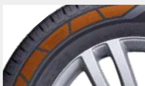
Prevents sidewall damage from the curb stone using low pressure conditions.
