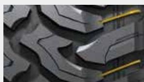
By connecting the tread and shoulder part, power through mud and soil condition and delivers improved high off-road traction.
