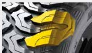
Stone ejectors protect the tread grooves against stone drilling and puncturing. Also shed the mud and stones from the tread grooves to maximise the grip.
